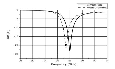
Figure 4.1. Simulated and measured S<sub>11</sub> of the single element MPA.
