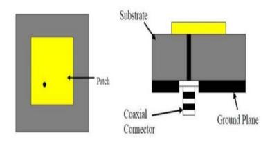
Figure 2.10. Coaxial / Probe Feeding [29].
