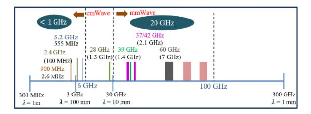
Figure 1.4. MmWave region of the electromagnetic spectrum
