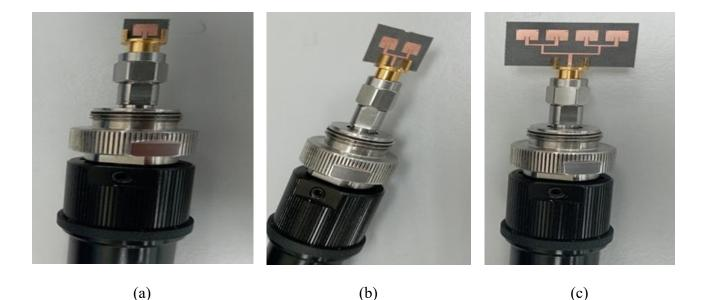
Figure 3.4. Fabricated (a) prototype of single element (e) prototype of  $1 \times 2$  elements (f) prototype of  $1 \times 4$  elements.
