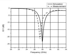
Fig. 3: The comparison of simulated and measured reflection coefficients at 28 GHz
