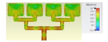
Figure 10. Surface current distribution of the MPA of 1×4 elements
