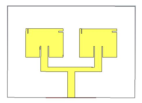
Figure 3.2. Geometry of the  $1 \times 2$  array element antenna at 28 GHz substrate size is  $10.3 \times 14.2$  mm.
