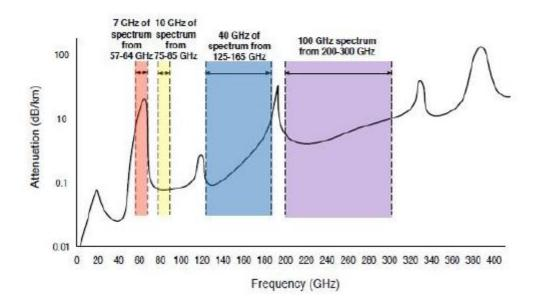
Figure 1.5. Average sea level atmospheric absorption at mmWave frequencies
