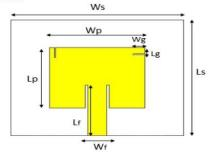
Fig. 1: Geometry of the proposed MPA at 28 GHz
