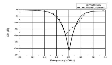
**Figure 4.7.** Simulated and measured  $S_{11}$  of the MPA array of  $1 \times 4$  elements.
