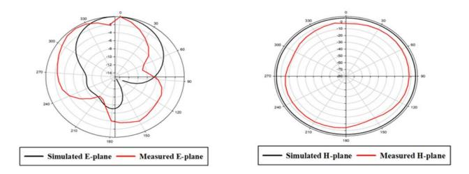
Figure 4.2. Simulated and measured radiation pattern of the single element MPA.
