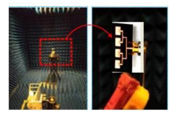
Figure 3.6. Far-field measurement setup.
