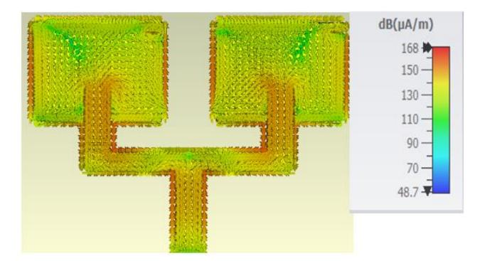
Figure 4.6. Surface current distribution of the MPA of 1×2 elements.
