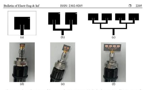
Figure 1. Design and prototype of the proposed MPA at 28 GHz (a) single element MPA, (b) MPA array of 1×2 elements, substrate size is 10.3×14.2 mm, (c) MPA array of 1×4 elements, substrate size is 14.3×26.2 mm, (d) prototype of single element, (e) prototype of 1×2 elements, and (f) prototype of 1×4 elements
