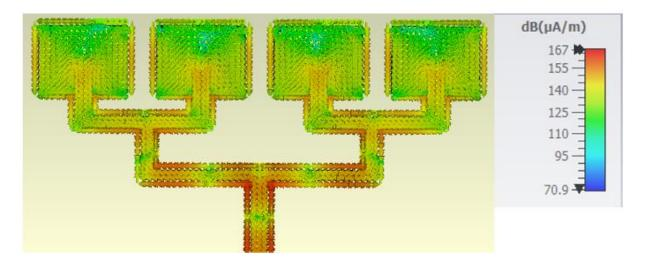
Figure 4.9. Surface current distribution of the MPA of 1×4 elements.
