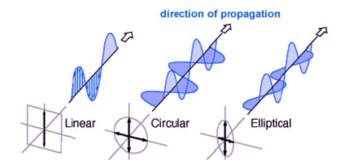
Figure 2.7. Polarization Linear, Circular, Elliptical.
