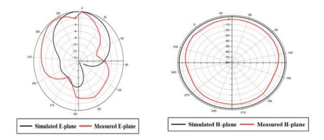
Figure 4.8. Simulated and measured radiation pattern of the MPA of 1×4 elements.
