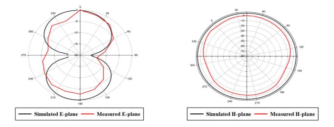
Figure 4.5. Simulated and measured radiation pattern of the MPA of 1×2 elements.
