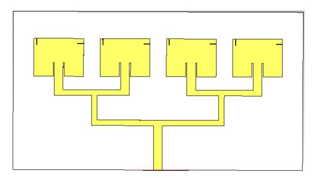
Figure 3.3. Geometry of the  $1 \times 2$  array element antenna at 28 GHz substrate size is  $14.3 \times 26.2$  mm.
