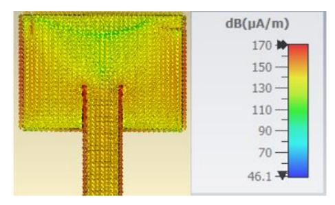
Figure 4.3 Surface current distribution of the single element MPA.
