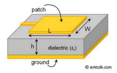
Figure 2.8. Structure of a Microstrip Patch Antenna [28].
