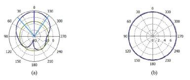
Figure 6. Radiation patterns of the MPA array of 1×2 elements (a) E-plane and (b) H-plane
