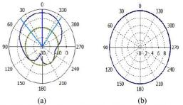
Fig 4: Radiation patterns at 28 GHz (a) E-plane (b) H-plane
