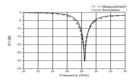
Figure 4.4. Simulated and measured S<sub>11</sub> of the 2-element array MPA.
