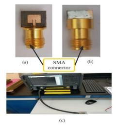
Fig. 2: Photographs of the (a) front view fabricated prototype (b) back view fabricated prototype (c)  $S_{11}$  measurement setup
