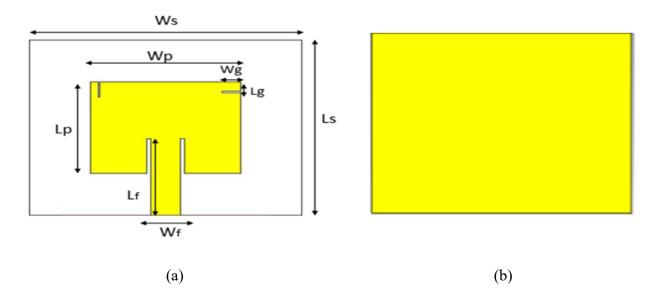
Figure 3.1. Geometry of the single element antenna at 28 GHz.
