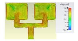
Figure 7. Surface current distribution of the MPA of 1×2 elements
