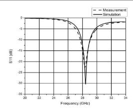
Figure 5. Simulated and measured S11 of the MPA array of 1×2 elements
