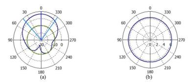
Figure 3. Radiation patterns of the single element MPA (a) E-plane and (b) H-plane
